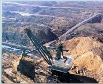
FIGURE 12.5 Some giant mining machines stand as tall as a 20-story building and can scoop up thousands of cubic meters of rock per hour. Note the pick-up trucks in the machine's shadow.
